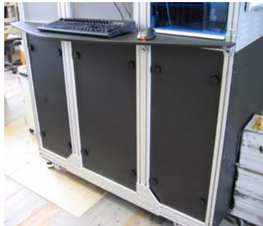
Figure 1. Remove front and back panels to access the paper path.
