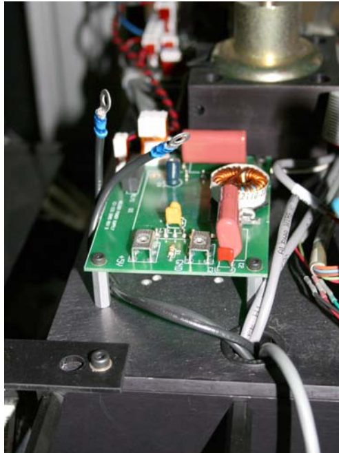
Figure 6. Push the cables down through the top of the Cut Weld Assembly.
